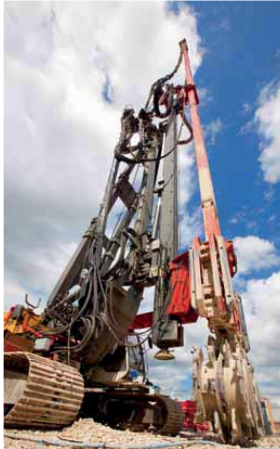
THE HYDROFRAISE XS is more compact than the standard model and can build diaphragm walls of less than 630 mm thickness.
